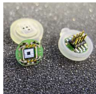
The sensor package for gas analysis has been designed to monitor fuel cells used for instance in transportation and rescue applications.
