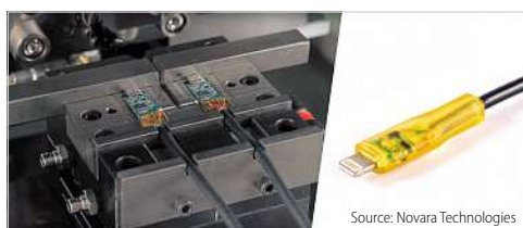
Encapsulation of electronic circuits and sensors in medical cable assemblies offers protection from accidental damage and tampering.
